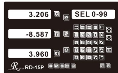
There are 100 feature memory available in RD-15P, they are feature 0-99 respectively, in this example, we are going to store this point parameters as feature 10, procedure are as follows
