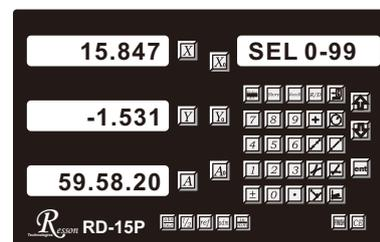
There are 100 feature memory available in RD-15P, they are feature 0-99 respectively, in this example, we are going to store this point parameters as feature 08, procedure are as follows
